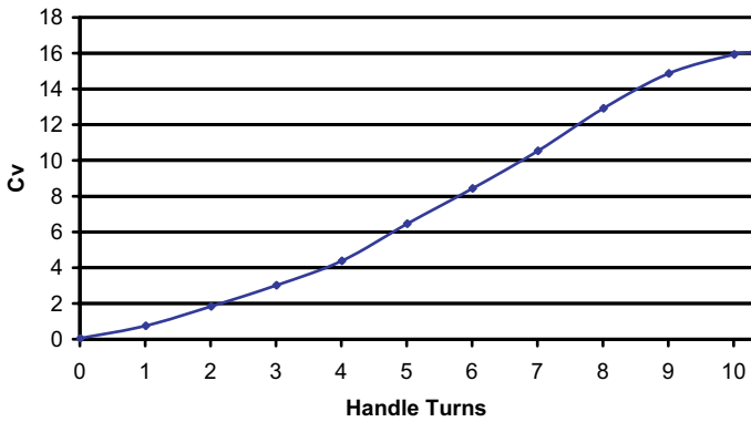
Cv vs Handle Turns for a 10K Throttle Valve with 5/8" Orifice
