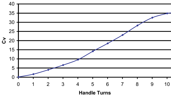
Cv vs Handle Turns for a 10K Throttle Valve with 1" Orifice
