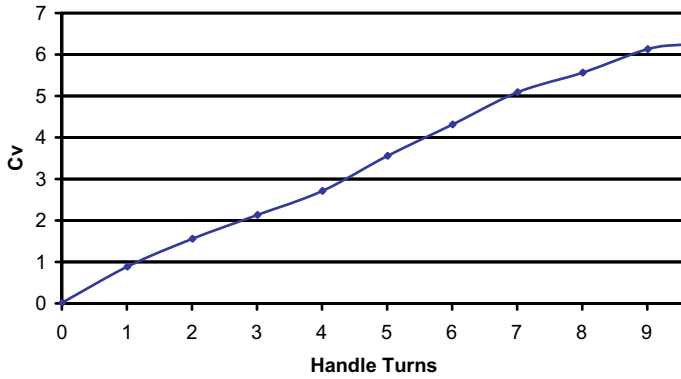
Cv vs Handle Turns for a 8H Throttle Valve with 7/16" Orifice
