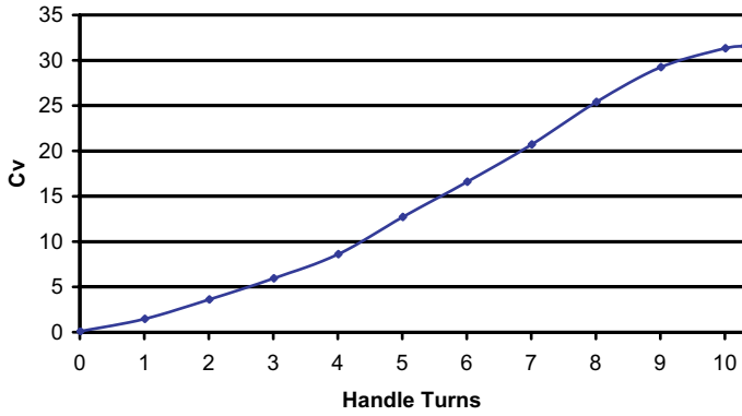
Cv vs Handle Turns for a 10K Throttle Valve with 15/16" Orifice
