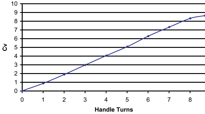
Cv vs Handle Turns for a 7G Throttle Valve with 1/2" Orifice
