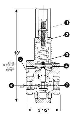
Pilot Materials Bronze B-62 Stainless Steel ASTM A743/CF8M
