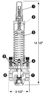
Pilot Materials Stainless Steel ASTM A743/CF8M
