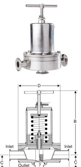
**Dimensions** (inches) Valve Weight Size В С D A Lbs 3/4" 3.29 8.50 1.50 5.70 6.58 19 5.70 8.00 1" 4.00 8.50 21 1.64 1-1/2" 4.24 10.5 2.53 7.25 8.48 41
