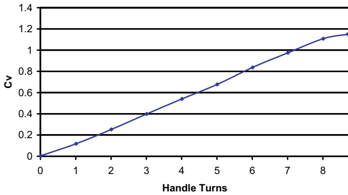
Cv vs Handle Turns for a 7G Throttle Valve with 3/16" Orifice
