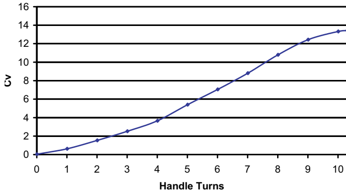
Cv vs Handle Turns for a 10K Throttle Valve with 9/16" Orifice
