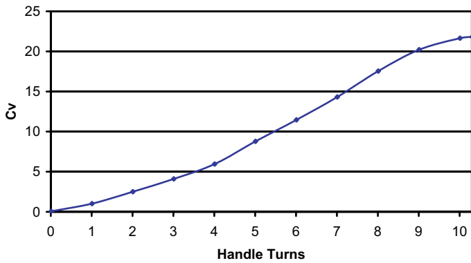
Cv vs Handle Turns for a 10K Throttle Valve with 3/4" Orifice
