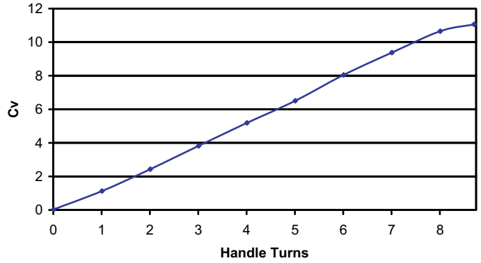
Cv vs Handle Turns for a 7G Throttle Valve with 9/16" Orifice
