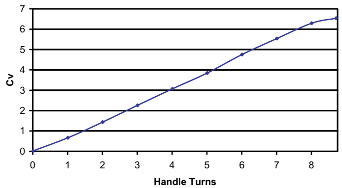
Cv vs Handle Turns for a 7G Throttle Valve with 7/16" Orifice
