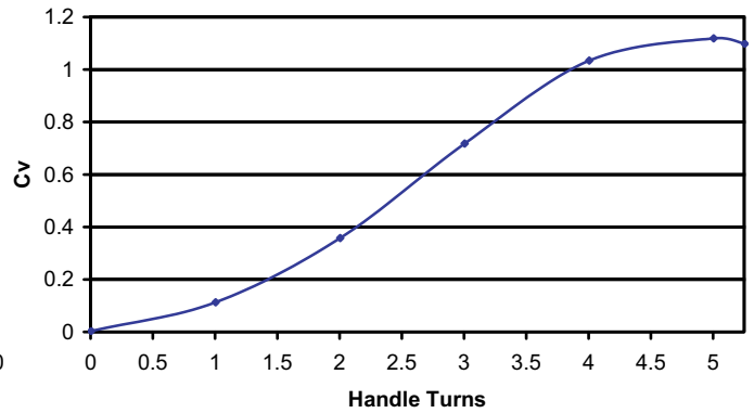
Cv vs Handle Turns for a 5E Throttle Valve with 3/16" Orifice
